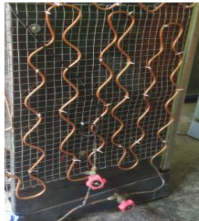
fig 5.1.2: Crimped Copper Condenser
